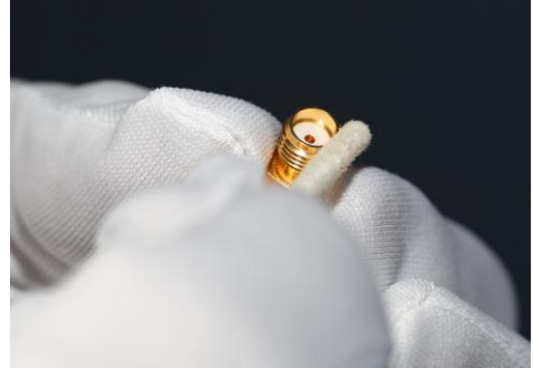
Figure 12 - Cleaning the thread
