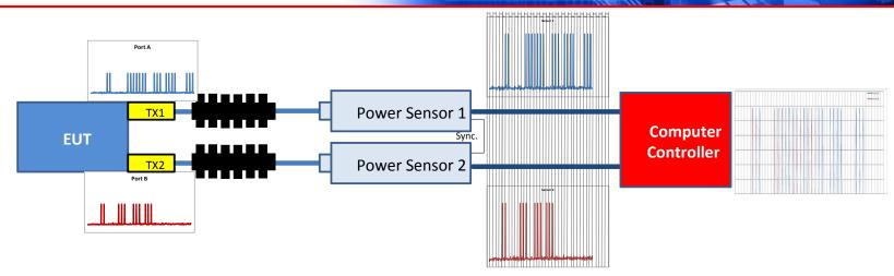
The multiple sensor measurements are combined in accordance with ETSI 300 328 and ETSI 301 893 The start and stop times of the individual burst must be recorded in order to determine the Power over the burst using the formula shown in the standard.
