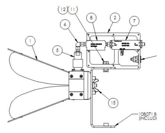
HPF filter used in series with Pre amplifier
